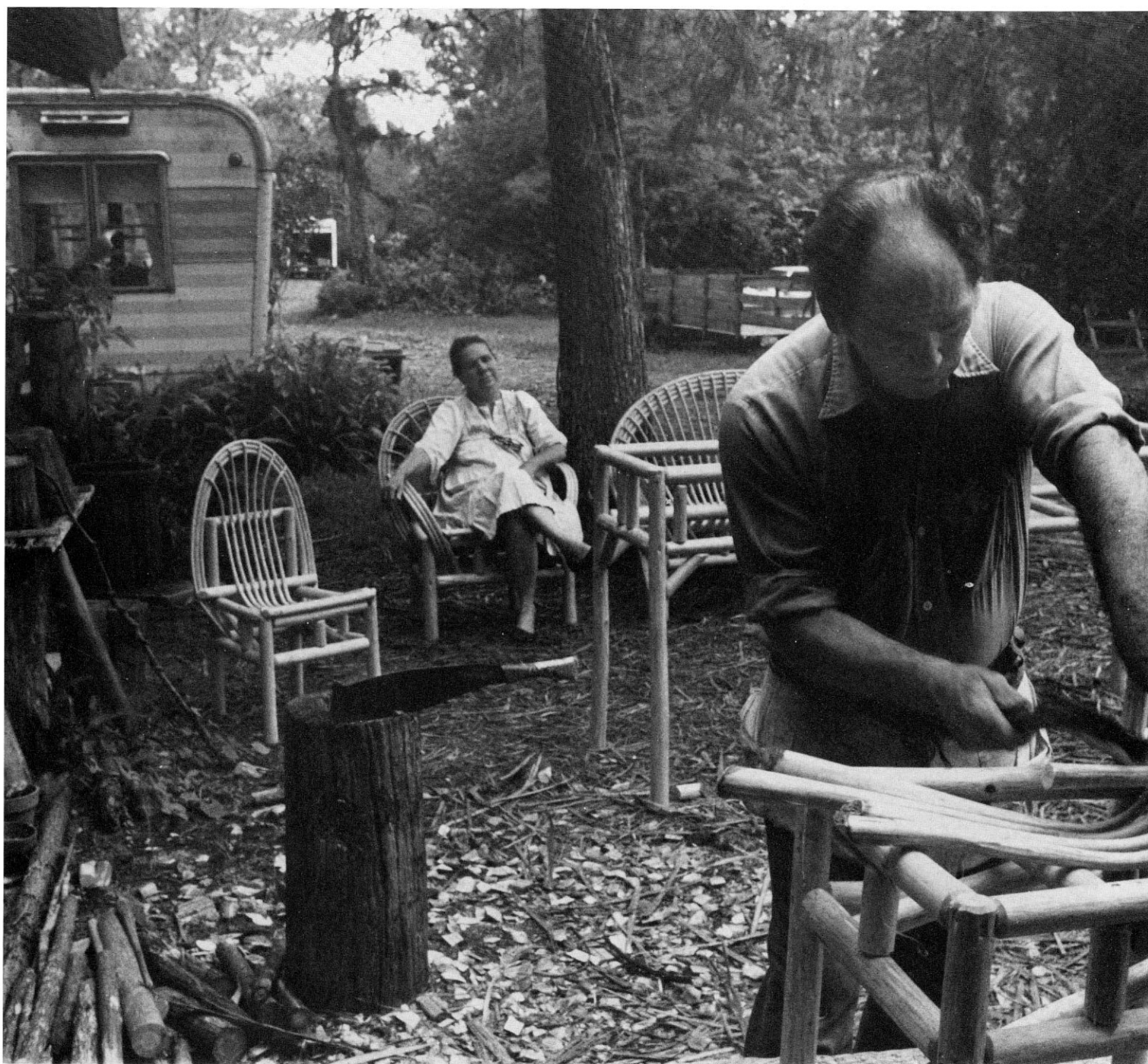
Betty Rudd looks on as Robert nails pre-shaped "benders" to the chair frame.
